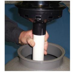
You CANNOT pull standpipe up to secure the valve. Pulling up can damage the laterals and cause sand to get sent back with water flow to pool.
