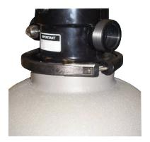
Make sure that the screws of the clamp are lined up with the seams of the tank. Tighten two screws on clamp a little at a time. Alternating from side to side so that both sides are tighten equally.
