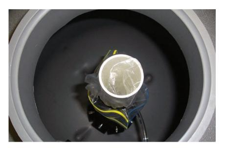
Clear plastic tube attached to standpipe is an air relief. As you are adding the sand
