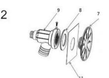
Attach #9 Water Flow Housing-outside of the pool, place #8 Double Sided Rubber Seal on Return Hole and #11 Pool Liner (not part of assembly),on the inside of the pool thread #7 Interface Plate into the Water Flow Housing
